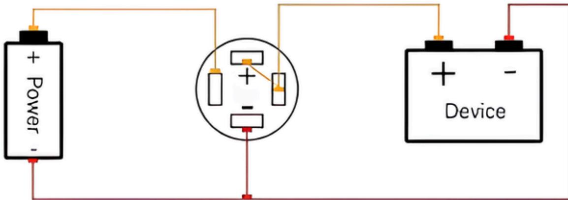
Press the switch, and the load will be powered when the switch light is on
